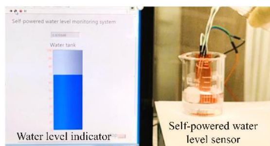
Fig. 1. Demonstration of a LabVIEW based self-powered water level monitoring system.
