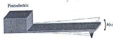
Fig. 2 Schematic diagram of external cantilever actuation mechanism by piezoelectric.
