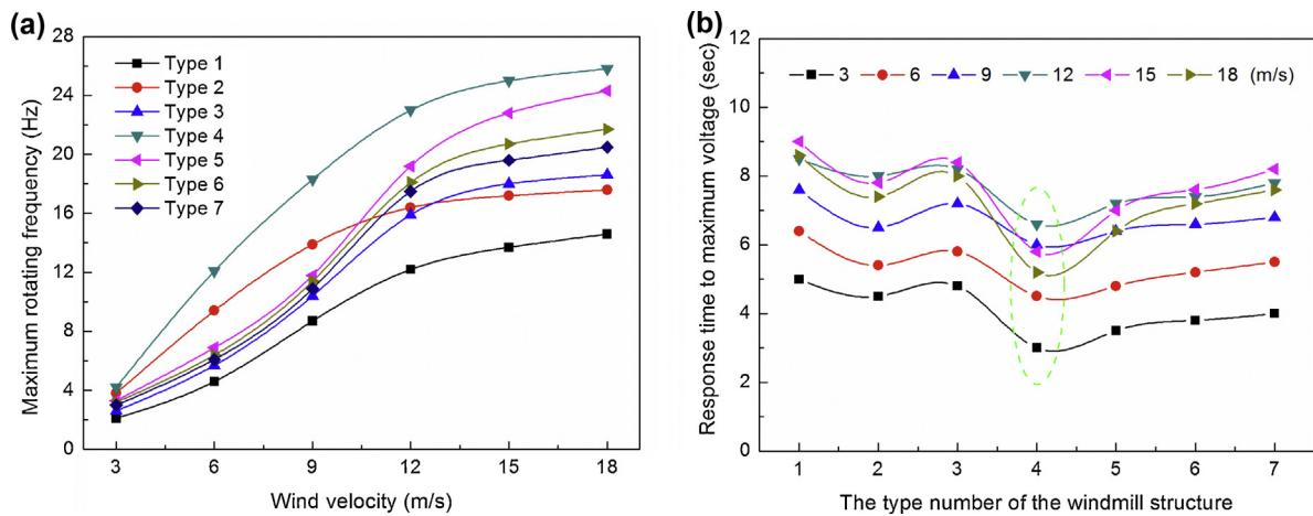
**Fig. 4.** The performance characterization for the 7 types of windmill structures. (a) The maximum rotating frequency versus input wind velocity. (b) The response time to maximum voltage under various input wind velocities.
