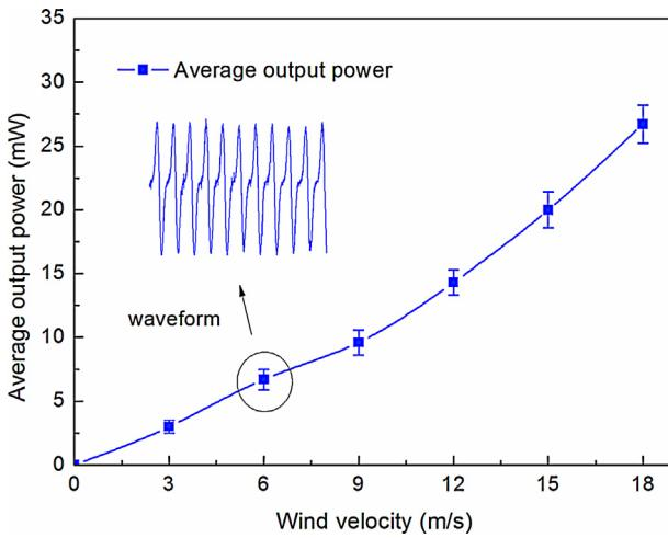
**Fig. 6.** The average output power of the windmill-structured energy harvester with various input wind velocities.
