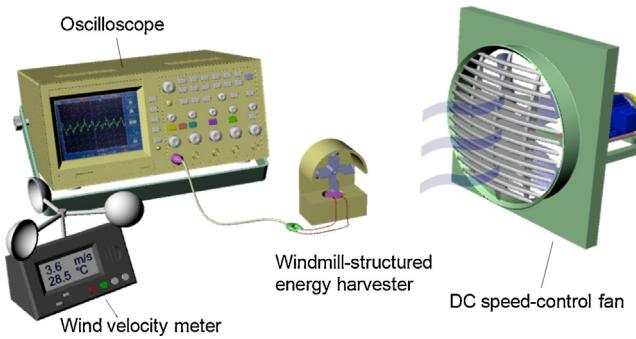
**Fig. 3.** The schematic of performance test setup.
