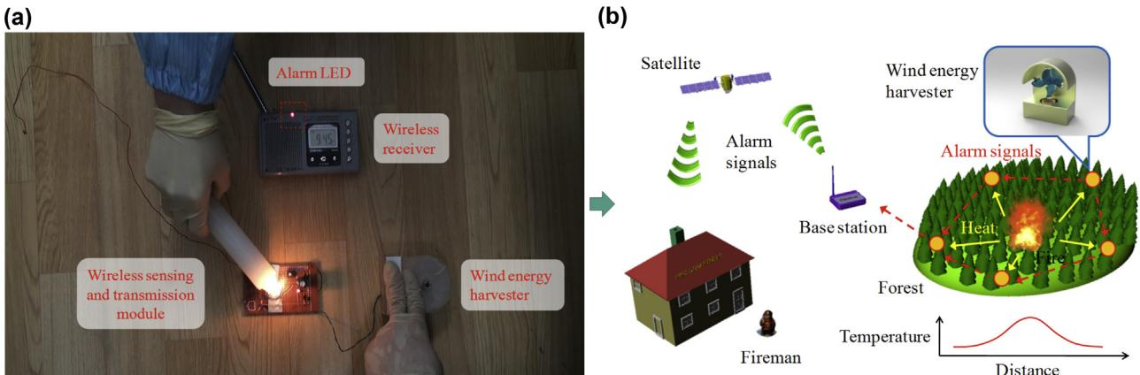
**Fig. 7.** (a) The experimental setup for windmill-structured energy harvester based fire monitoring and alarming system. (b) The schematic of wireless forest fire monitoring by the windmill-structured energy harvester.
