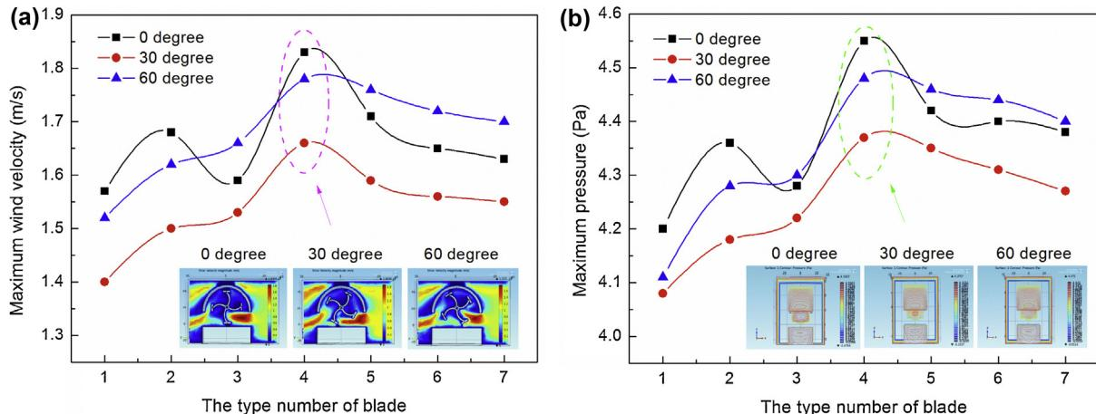
**Fig. 2.** COMSOL simulation results on the (a) wind velocity distribution and (b) pressure distribution for different types of blades. The input wind velocity is 1 m/s, and the blade is rotating at angles 0°, 30°, 60°, respectively.
