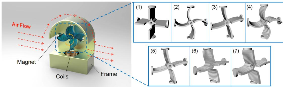
**Fig. 1.** The working schematic of the windmill-structured energy harvester with various designs of the replaceable windmill structure.
