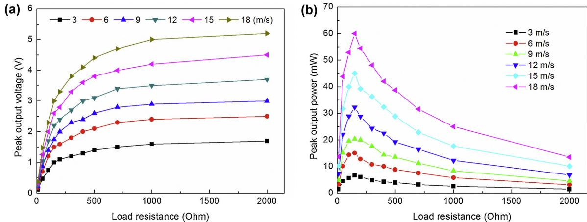
**Fig. 5.** Resistance optimization: (a) Peak output voltage versus load resistance for different input wind velocities. (b) Peak output power versus load resistance for different input wind velocities.
